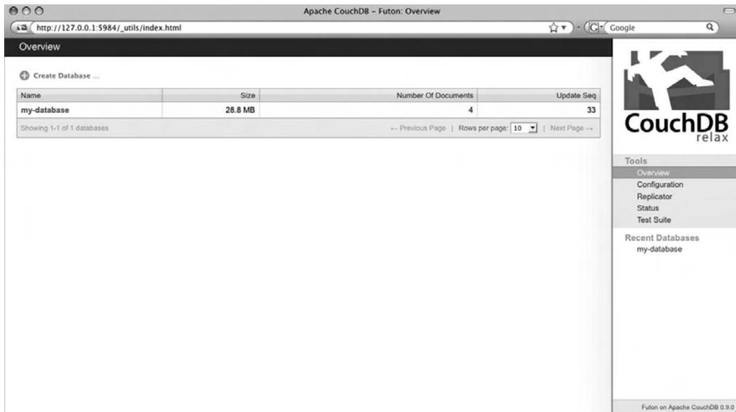
Figure 12-14. A database in need of compaction
