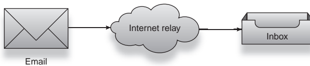
Figure 1.1 Email is composed locally, delivered across an internet relay, and received by an inbox.
